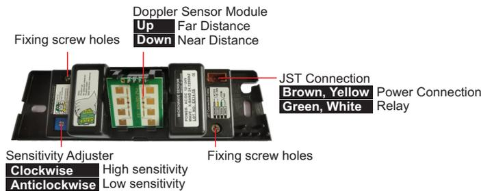
1. Place the sensor in the proper position, remove the burrs completely of the cable hole, and open the mounting plate.
