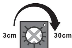
Clockwise direction adjustment, distance becomes more far, counterclockwise direction adjustment, distance becomes more near. The max sensing distance is 30cm.
